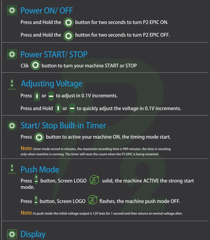
Voltage, Capacity and Timer display alternately every 5 seconds under the machine working condition.
